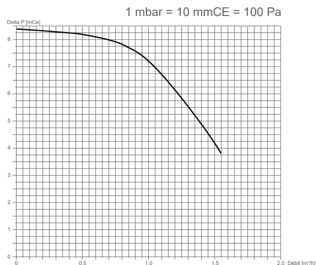
fig. 2 - Available hydronic pressures and flow rates
